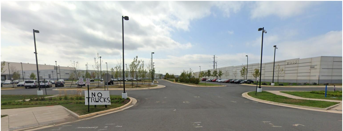
An example of parking area light poles that are higher than needed, especially in an area where trucks are not permitted. Waxpool Rd - Google Maps
